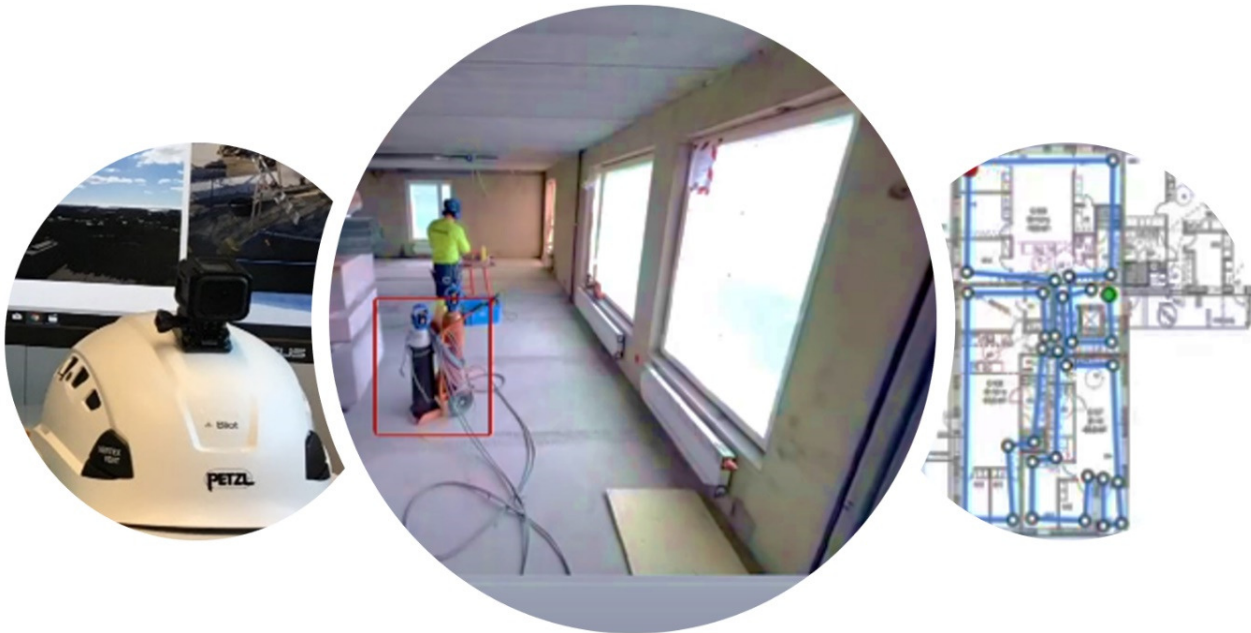
Figure 3 – Remote Supervision – ‘ Be There ’ with 360 camera feed, pick a location from the ‘snail trail’ and look around with ease and HD clarity. Take Measurements, Review Progress, Delegate Tasks and Note Conditions from any day in the site history.
